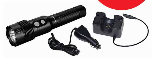
The Flashlight is made of a lightweight durable aircraft-grade aluminium. It has a 3.7V Li-lon battery, with a runtime of up to 120hrs, which runs an LED with a Maximum Lumen output of 1000 and has a lifespan of 50,000 hrs. The LED has a range of up to 950 feet and the flashlight is impact resistant and waterproof up to 2M deep.
