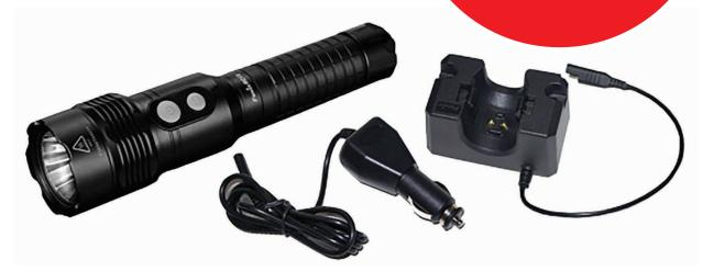
The Flashlight is made of a lightweight durable aircraft-grade aluminium. It has a 3.7V Li-Ion battery, with a runtime of up to 120hrs, which runs an LED with a Maximum Lumen output of 1000 and has a lifespan of 50,000 hrs. The LED has a range of up to 950 feet and the flashlight is impact resistant and waterproof up to 2M deep.
